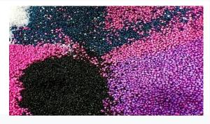
The plastic waste is turned into granules and used to make the road surface
